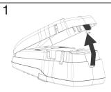
Press the open cover lock at the top of 0m and pull upward.
