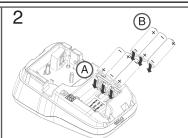
Load six new AA alkaline batteries (LR6: not included) or fully charged nickel metal hydride batteries (HR6: not included) to ensure that the polarity of these batteries is in the right
